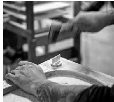
A wedge lock joint used in the Papa Bear Chair , the Upholstered Peacock and the Stool to make the strongest possible connection between the legs and the frame.
